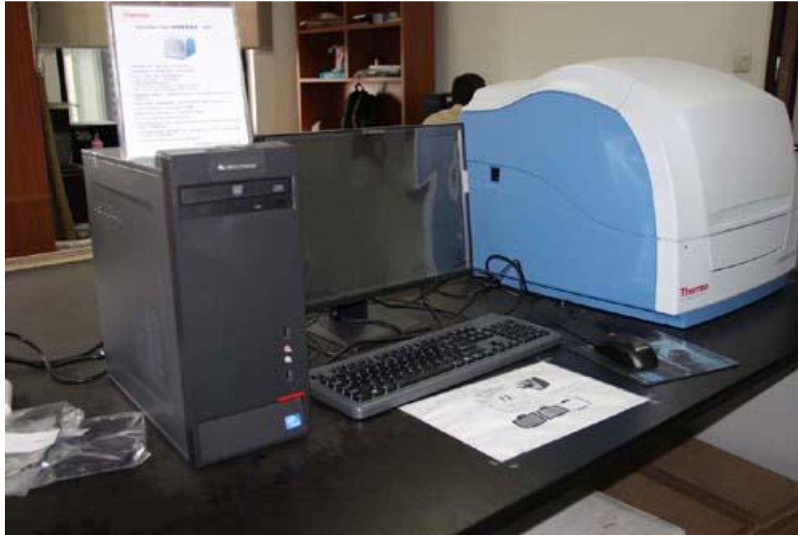
Multimode plate reader (spectrophotometry, fluorescence and luminescence)
